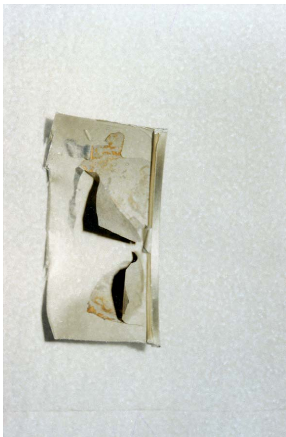
Fig. 5. Enamel adhesion failure on internal walls of defective (F) cans.
