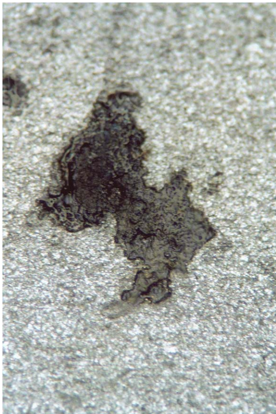
Fig. 4. Sulfide staining on internal walls of defective (C) cans using the “cysteine” test.
